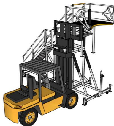
Figure 3 – Joining the platform to the base section
